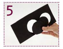
Now make the cam and a cam follower. Draw the shape of the cam and the cam follower on the thick foam sheet, and then cut them out. The cam should be about 6cm in diameter and the cam follower a little bit bigger. Tip: Cut these smoothly for the best motion
